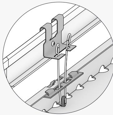
Simply run your torsion spring through the Spring Clip and Adapter, and push up to snap your panel into place!
